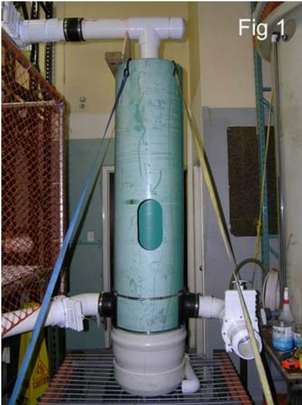
In this experiment the system was operated at two different continuous flow rates: 80gpm and 100 gpm. These rates were measured through the use of dual, in-line flow meters, which had been calibrated using accepted catch-and-weigh techniques.
