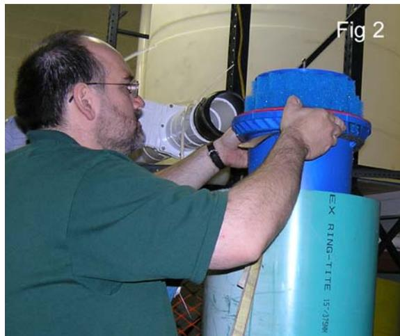
of the filters ability to remove free and emulsified oils and grease without the interference of suspended solids. This a more conservative approach as sediments readily bond with oils and grease which then get trapped in the filter by mechanical means. Varying the TSS concentration and particle size distribution could affect oils & grease removal rates by some unknown percentage.
