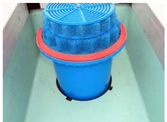
Once the Tabs fall through the slots, continue turning firmly in a Clock-wise direction until the Tabs contact the STOPS. The Cartridge is now installed.
